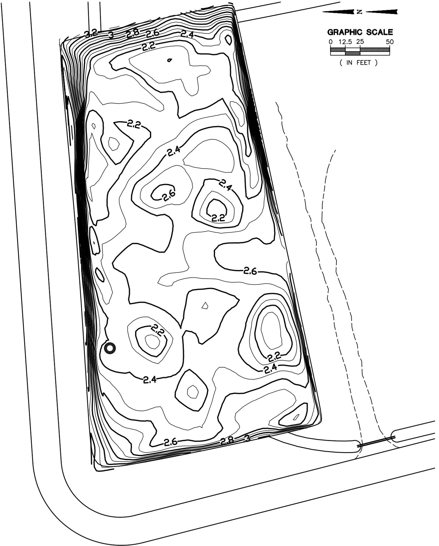
Figure 2-3. Elevation Contours for the Dry Detention Pond (Ft. NGVD).
